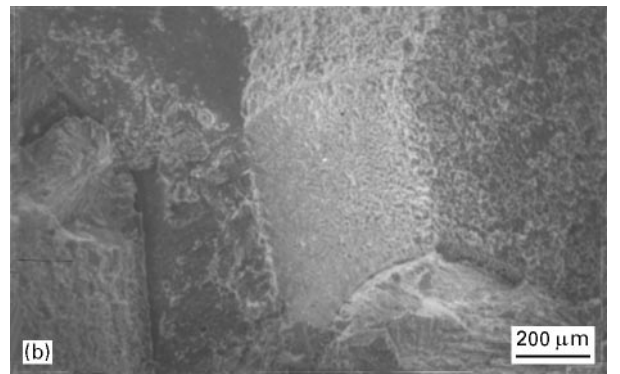
Figure 10 Typical failure modes in as-received elevated-temperature toughness specimen (a) planar slip/cleavage in \alpha_2 grains and plastic stretching of \beta phase; (b) intergranular fracture; and (c) profuse microcracking.
