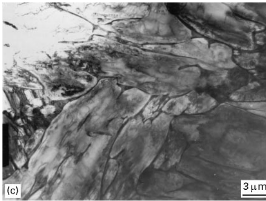
Figure 11 TEM Images of typical crack-tip and undeformed regions in as-received material. (a) Interfacial dislocations in crack-tip region, (b) straight and bowed dislocations in crack-tip region, and (c) low dislocation density in undeformed material.
